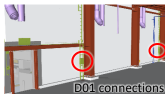
Figure 28: E02 Connectors/ Conventional (Installation) Power Network (230V /400V). See 0 for details
