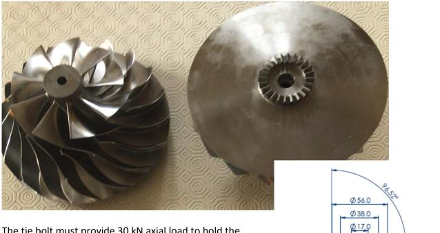
The tie bolt must provide 30 kN axial load to hold the wheel in place – this can be achieved using an Inconel tie bolt and high tensile nut with an M10 thread.
