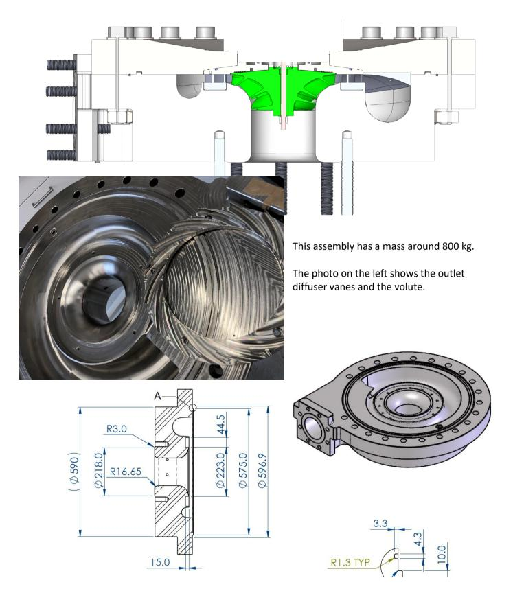
The above parts fit into an existing skid which contains flow measuring, valves and process instrumentation. The image below shows the volute mounted on the skid using anti vibration rope mounts.
